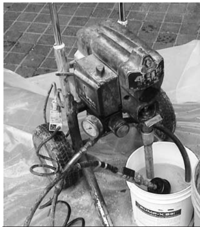
PHOTO: Airless sprayer, adapted for pumping of PUMP-X53i. Spray gun was removed and replaced with a ball valve and adaptor, bushed down to 1/8" diameter tubing. A rubber seal, set 2-3" above end of tubing, prevents grout from running out of injection port.
