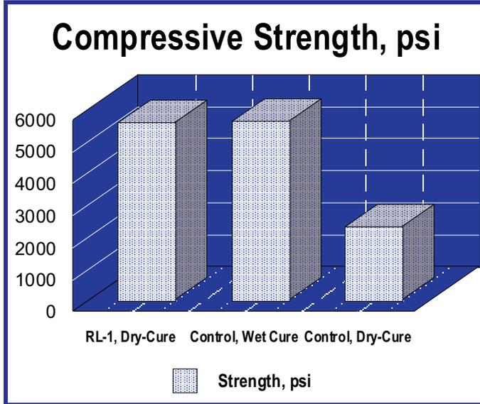
mortars, patches and plasters to which they are applied. Compressive strength is determined by the mix design of the cement-based material to which the latex modifier is added. Latex modifiers simply assure that mixes will reach the intended design strength *without the necessity of wet curing*.
