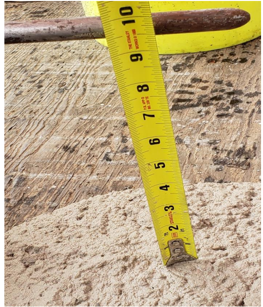
Step 3: Measure slump according to ASTM C143/C143M.
