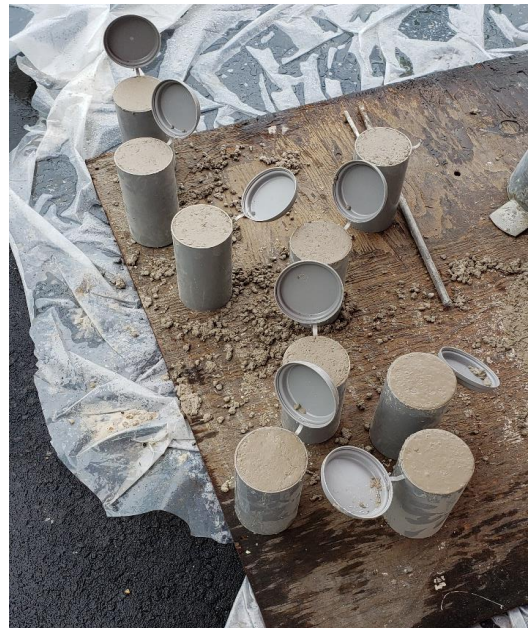
Step 4: Cast cylinders for compressive strength testing according to ASTM C31/C31M.
