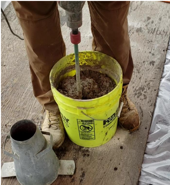
Step 2: Mix for 4 minutes using a 250-400 rpm drill mixer.
