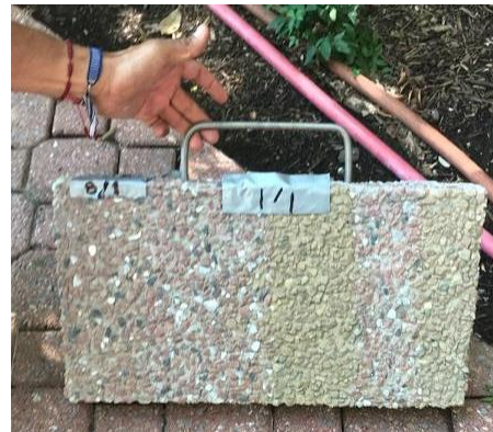
Photos: Mockup panel, above. Custom-matched exposed aggregate repairs utilizing REPLIC-8, left. The two scaffold drops on the right are in progress. The four drops to the left are completed. Courtesy Atlantic Co. Of America.
