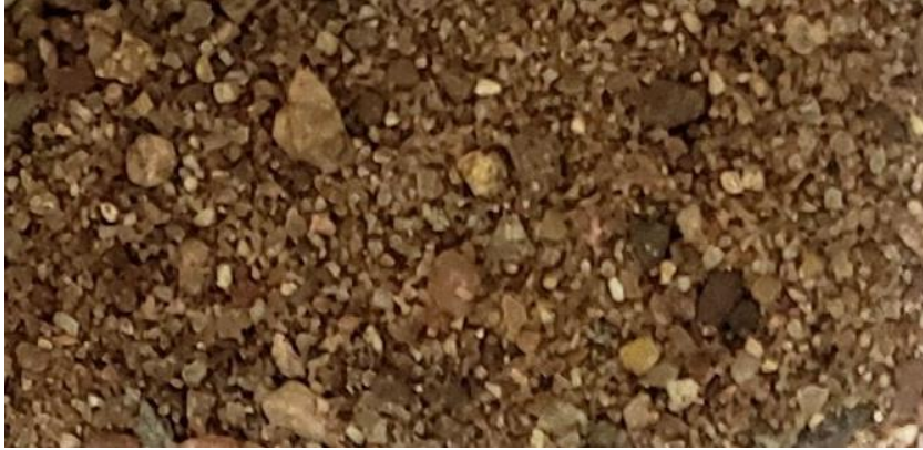
Photo: Natural Connecticut Valley brownstone sand used in Custom System 45 Type SD Brownstone repair mortars. Aggregates that are close to the color and composition of the host stone provide better detail and long-term color retention than simple pigmented cement matrices. Sands can also be custom-sieved to provide better texture match to each individual host stone.
